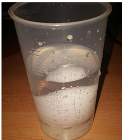
Figure 2 – Determination of egg volume according to Archimede's principle
