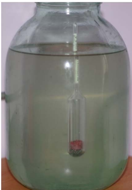
Figure 3 – Salt brine with a density of 1,085 g/cm 3
