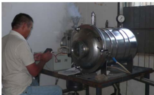
Fig.2 – Arrangement for sublimation during drying condition process
