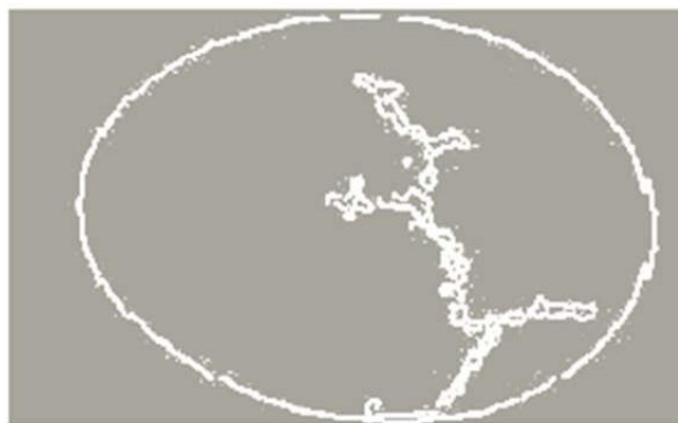
Figure 4 - Result of the definition of a crack based on the AI SUSAN-detector.
